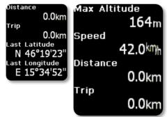
If the RC T3000 is powered OFF all this data (except last known latitude and longitude) will be reset. Last known latitude and longitude will be stored until "init memory" is done in Setup.
