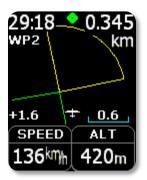
The GPS triangle task is a complex navigation procedure which guides the pilot from the start point around 3 turn points until the finish line. The task can be created manually or imported from the SD card. On this page the pilot can find basic information on how to approach the next TP on the task.
