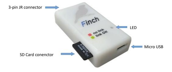
Figure 1: The Finch Serial module.
